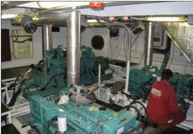
Machinery spaces with 2 X L136TI and 1 AD136 in "Seaclear"
